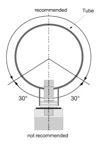
Please install the sensor only in the recommended area like you can see in the picture. A upside down installation is not permitted. Please consider that the distance to the vertical level must be >30°.
